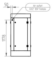
The compressor can be installed on any level floor capable of supporting it. A dry, well ventilated area where the atmosphere is clean is recommended. A minimum of 600mm at the rear, the top and all sides of the machine is recommended for adequate service access and ventilation.
