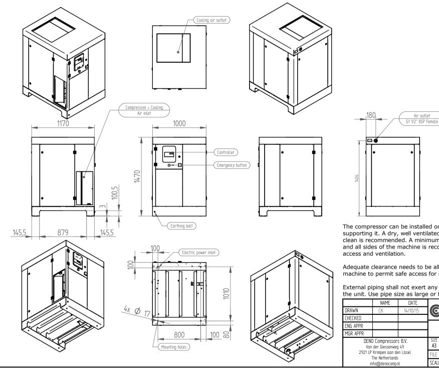
The compressor can be installed on any level floor capable of supporting it. A dry, well ventilated area where the atmosphere is clean is recommended. A minimum of 800mm at the rear, the top and all sides of the machine is recommended for adequate service
