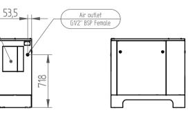
The compressor can be installed on any level floor capable of supporting it. A dry, well ventilated area where the atmosphere is clean is recommended. A minimum of 600mm at the rear, the top and all sides of the machine is recommended for adequate service access and ventilation.
