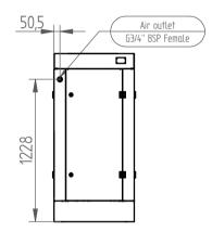
The compressor can be installed on any level floor capable of supporting it. A dry, well ventilated area where the atmosphere is clean is recommended. A minimum of 700mm at the rear, the top and all sides of the machine is recommended for adequate service access and ventilation.
